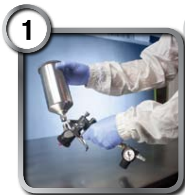
1 Remove existing cup from spray gun.
