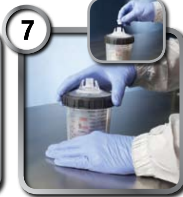
7 Position locking collar onto the 3M™ PPS™ cup/liner and turn until tight. Insert sealing plug prior to shaking.
