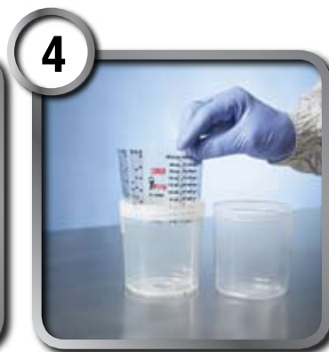
4 If not using a scale to measure, insert 3M™ PPS™ Mix Ratio Film into cup before inserting liner in order to measure the paint according to paint manufacturer's guidelines.
