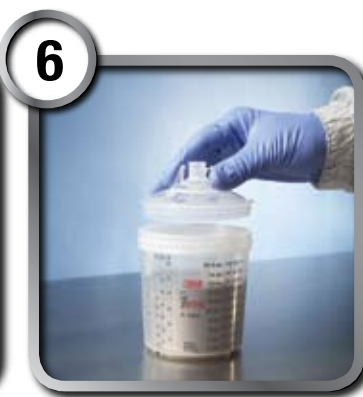
6 Take a lid (with built-in filter) from wall dispenser and snap into the 3M™ PPS™ cup/liner.
